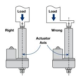
Loads should act along the axis of the actuator. Off-center loads may cause binding and lead to premature unit failure.
