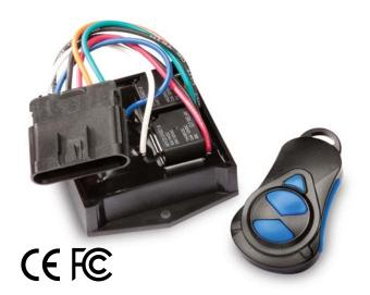
Warner Linear's wireless actuator control can be used to remotely control a 12 or 24VDC actuator up to 100 ft. away. It can be used with our standard line of P1 end limit controls. The unit is offered in a single and dual actuator output for the 12VDC unit. The 24VDC unit is only available with two actuator outputs. All models have a manual override feature to operate the actuator without a remote. The wireless system is an RF design operating at 915MHz.
