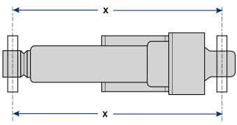
Mounting pins must be parallel to each other as shown above. Pins which are not parallel can cause excess vibration or actuator binding.
