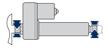
Do not attempt to mount M-Track actuators by the cover tube. The tube is not designed to support the forces required for tube mounting.
