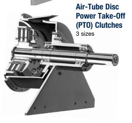
Air-Tube Disc Power Take-Off Clutches provide dependable trouble-free performance on indirect drives with large overhung loads on engines of 250-700 HP. The Wichita design isolates the side load from the engine's crankshaft for long service life. Simple air controls can be utilized to remotely control the clutch as well as the throttle. Wichita PTO's have been successfully used for oil field, construction and marine applications.
