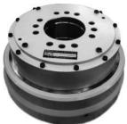
The Model HC(D) clutches are provided with an internally splined outer drive ring for bolting to the users driving or driven member. The clutch can also be supplied without an external drive ring to allow for customers to incorporate the external drive spline within a component of their own manufacture. This possibility enables designs where minimal axial space is desirable, by allowing the clutch to fit within the customers driving or driven component.
