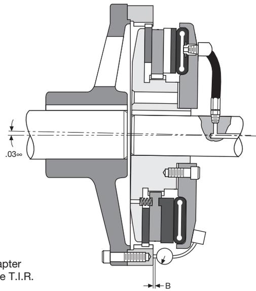
Rotate Driving Adapter Ring 360 to determine T.I.R.
