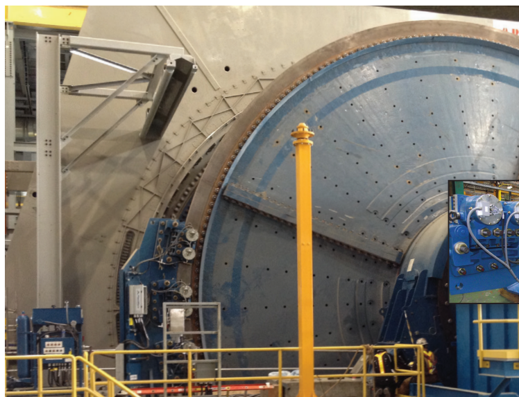
One of two VMS-DP brake stations supplied for the 12.2 m dia. gearless SAG mill
