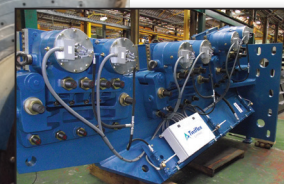
One of two VMS-DP brake stations supplied for the 12.2 m dia. gearless SAG mill
