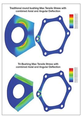
Figure 2: FEA stress comparison of a typical round bushing and a  $Tri-Bushing^{TM}$ .
