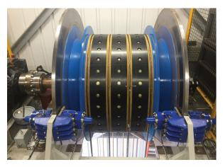
To meet a mine's hoist emergency stopping and parking application requirements, Twiflex provided Series VKSD spring-applied, hydraulically released, dual-spring caliper brakes.
