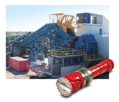
A major international metals recycler was experiencing problems on their shredders due to universal joint damage caused by excessive torque generated during rotor jams. Repeated repair and replacement of the damaged universal joint cross and bearings required costly downtime.
