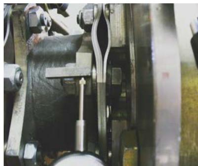
FIG. 20- COUPLING AT 500% OF RATED TORQUE
