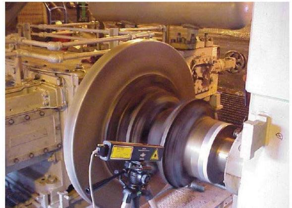
FIG. 32- TORSIONAL LASER VIBROMETER USED TO MEASURE TORSIONAL VIBRATION AT THE COUPLING (COURTESY OF BETA MACHINERY)
