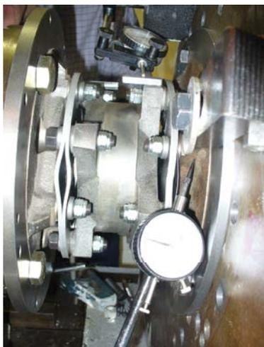
FIG. 19- COUPLING AT 267% OF RATED TORQUE
