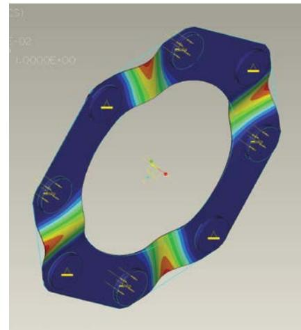
FIG. 28- NONLINEAR DISC FEA RUN SHOWING BUCKLING IN COMPRESSION LEGS. TENSION LEGS ARE FLAT
