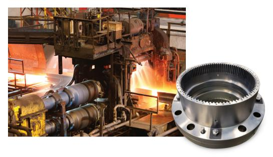
A major steel manufacturer needed a large replacement gear coupling as part of an upgrade for a roughing stand drive at one of its U.S. mills. Positioned on the low-speed, high-torque shaft between the gearbox and pinion drive, the gear coupling rotates at approximately 10 RPM. The goal was to ensure that the new coupling was capable of transmitting the new, higher torques.
