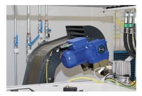
By adopting an intelligent electronic control, it's possible for the operator to set a flexible, yet precise overload torque and constantly monitor performance.
