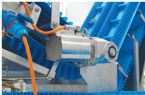
Stainless steel geared motors are often selected as they meet all application requirements without the need for further coatings.
