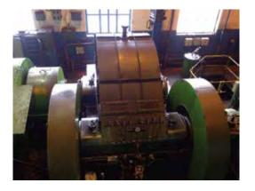
manufactured by Bibby, now part of Altra, so we asked if its coupling division would be able to help with a replacement. It was able to use the original design to manufacture a custom coupling which matched our criteria exactly."
