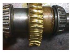
Chemicals found in many lubricants with EP (Extra Pressure) additives will soften the bronze worm gears and lead to rapid wear of the gear tooth structure.
