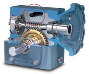
Pressure relief devices such as Boston Gear's unique PosiVent<sup>®</sup> system reduce seal strain and also eliminate the need for breather vents. This is especially important in washdown applications where breather vents can allow washdown solutions and water to get inside gearboxes. There, they breakdown lubricant, cause premature wear, and ultimately lead to unpredictable failure.
