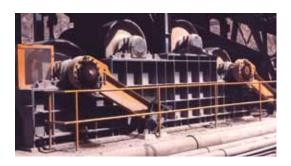
The torque arm is a simple device utilized on an array of industrial clutches and holdbacks with torques ranging from a few inch pounds to a million foot pounds. While very basic in design, when mounted incorrectly, all torque arms will yield the same negative result: costly unit failure and associated downtime.
