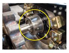
The compact 10 in. diameter FSO units fit within the existing hardware and the small space available. The sprag clutch is engaged for the up-mountain portion of the trip, preventing any roll-back of the passenger coach. For the down-mountain leg of the trip, the clutch is disengaged to allow downward movement.
