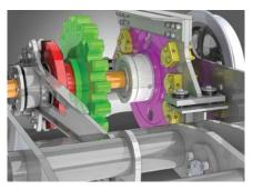
There are 12 hydraulic caliper brakes that hold the clutch rotor stationary when applied. To engage the clutch, the brakeman flips a valve which applies hydraulic pressure to the brake calipers, preventing the sprag rotor from rotating.
