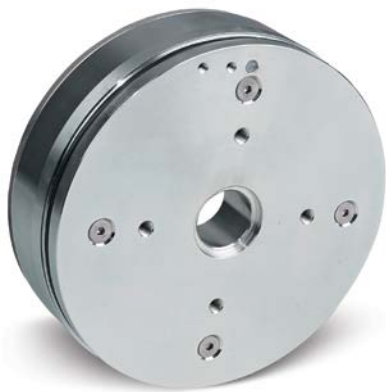
Compact Matrix Model 4PMB070 operator-controlled, variable torque permanent magnet brakes have a 190 Nm (140 lb.ft.) static torque rating and 150 Nm (110 lb.ft.) dynamic torque rating.
