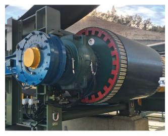
Dual RDBR 300 models with 70 kNm torque per unit are installed on the 1800 mm (5.9 ft.) wide, 3,050 m (1.9 mile) long drift conveyor at the Moolarben mine that transports coal from the longwall system underground to the surface. The inclined conveyor features an 80 m (262 ft.) lift and has a capacity of 4,500 tph.
