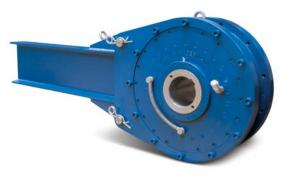
Stieber's self-contained, externally mounted RDBR-E lowspeed torque-limiting/ load-sharing releasable backstop features a power-dense, compact footprint. A fully bearing supported multi-disc brake provides the torque limiting function.
