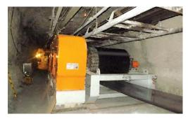
The brake disc diameter needed to be relatively small since space was very limited in the underground installation area.
