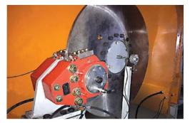
The Model BSFH 520 spring-applied, hydraulically-released, dual-spring caliper brakes with 160,000 N braking force, each act on a 50 in. x 1.25 in. standard steel brake disc.
