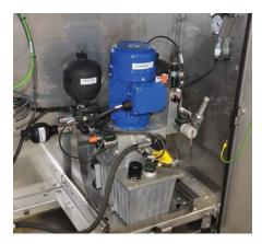
All Svendborg power units are designed and manufactured in-house to ensure compatibility with other Svendborg braking system components. Units are equipped to monitor oil level and temperature, motor and pump function, and system pressure.
