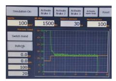
Remote access and touchscreen for setup and monitoring. The control utilizes different communication ties plus different communication protocols. Authorized users can easily access and change the parameters inside the control, such as defining a parking sequence or pre-setting a stop time.
