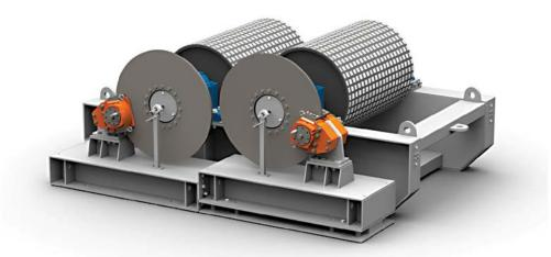
The new braking solution is used on the final two downhill longwall panel conveyors. Each conveyor is approximately 14,500 ft long with 725 ft of drop from tail to head. The 54 in. wide conveyor belt is driven by two 300 HP regenerative ABB VFDs, while operating at a speed of 630 ft/min. to move 1200 -1800 tph of coal.
