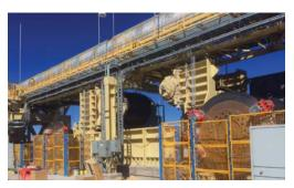
The entire four-flight, direct drive OGP1 conveyor system spans 10,632 m (6.6 miles) in length with the largest section being 3,942 m (2.4 miles) long.
