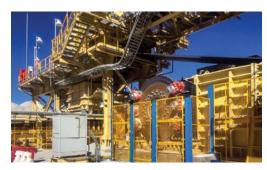
Groupings of six Model BSFB 650 spring-applied, hydraulically-released, dual-spring caliper brakes, acting on 2.7 m (8.8 ft.) diameter steel brake discs, serve as on/off holding brakes at the head of the various OGP1 conveyor sections.
