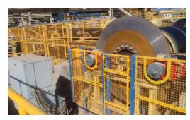
Pairs of Model BSFB 650 spring-applied, hydraulically-released, dual-spring caliper brakes, acting on 2.7 m (8.8 ft.) diameter steel brake discs, are positioned at the tail of the various OGP1 conveyor flights.
