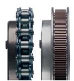
Roller Chain (left) and synchronous belt.
