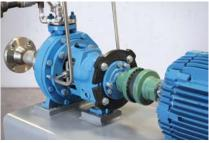
A size 7 TB Woods Sure-Flex Plus coupling was able to be installed instead of a larger size 8 coupling on this small Group 1 Summit/GPM ANSI pump unit. By utilizing the smaller coupling, the overall package length was reduced allowing for a smaller baseplate footprint.
