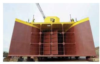
Designed to generate power in nearshore estuaries, the Neptune Proteus 1000 is controlled by a pair of Twiflex VKSD-FL caliper brakes and hydraulic powerpacks.
