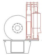
Twiflex GMR-SH-15 Brake Torque 11900Nm
