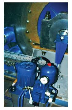
Typical Emergency Braking System showing calipers and hydraulic power pack
