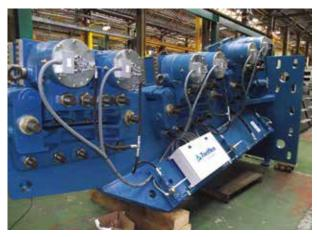
One of two VMS-DP brake stations supplied for the 12.2 m diameter gearless SAG mill.
