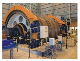
Twiflex provided parking brakes for use on mine hoists at the Nkana site of Mopani Copper Mines in Zambia.
