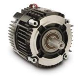
substitute for brut force. If you have a modest cycle rate, say 10 cycles/min, your cycling motor application may be enhanced by a high performance dynamic-cyclingpermanent-magnet-motor-brake module (a Warner EM-20-MBFB or FBB). It takes half the heat out of the motor and drive, dissipating it in the brake and provides long life dynamic stopping and no-power holding.
