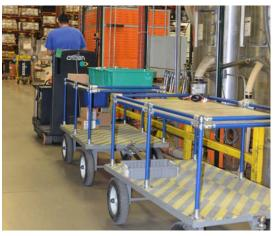
All raw materials and finished goods at the plant are delivered and retrieved utilizing a unique tugger train system that cycles through the plant every two hours.
