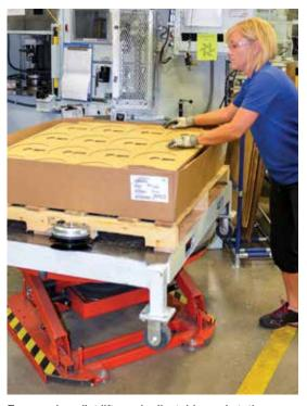
Ergonomic pallet lifts and adjustable workstations are utilized throughout the facility to provide an added measure of convenience and safety for associates.
