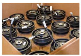
A variety of electromagnetic clutches and brakes, including PTO clutches and brakes for use on consumer and commercial lawn tractors, agriculture equipment and diesel engines are manufactured at the new plant.
