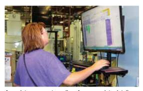
Associates now enter cell performance data details directly into an electronic visual management system for automated summation of near "real time" performance data. Large monitors, positioned next to the cells, display color-coded data for easier viewing by team leaders and supervisors.
