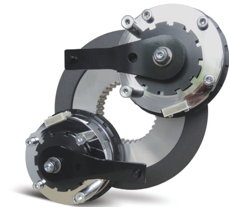
Figure 1: Warner Electric developed this custom brake because standard braking systems could not meet the elevator's difficult speed, energy, and dynamic torque constraints.
