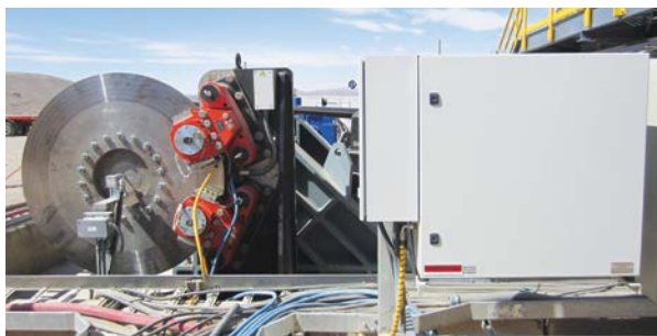
A complete Svendborg engineered brake system package, installed on a copper mine conveyor, consists of two BSFH 520 caliper brakes (red) and disc, a hydraulic power unit and a soft braking control (housed in two adjacent gray boxes on right).
