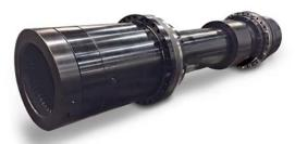
This 10' long, 23" diameter custom Ameriflex coupling features specific split retaining rings on both the pump and gearbox end hubs, multiple convoluted diaphragm pack flex elements at each end, and a special spacer configuration for added stiffness in this dual output application. An integral indexing/timing device aligns the coupling with the mixing blades of the polymer pump.
