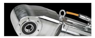
The IE4 super premium efficiency stainless steel geared motor is designed with surfaces which slope by at least 3° to prevent the formation of dirt deposits and allow the run-off of cleaning agents and water. Stainless steel construction eliminates the risk of the hygiene rating becoming compromised in the event of an impact or over prolonged periods of use in heavy washdown environments.
