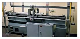
Detent/piston designs are routinely tested for 2 million cycles utilizing Kilian's unique Radial Bearing Durability Test Machine. The machine features a variable speed/variable distance precision-guided table and custom-designed fixtures that allow for testing multiple detents simultaneously.
