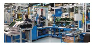
Manufacturing upgrades include a new production line divided into two new work cells. The primary work cell allows for semi-automatized assembly utilizing conveyors. Components and brakes are traceable via bar codes. Visio software is used for component presence and profile detection. A slaved system has also been incorporated for screwdrivers, di-electrical tests, etc.
