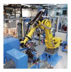
A new, multi-station robotized cell is also incorporated into the production process to provide friction disc burnishing, static torque adjustment, electrical adjustment, dynamic torque measuring, and component crimping to secure the adjustment. All production parameters are stored in a custom software program developed exclusively for Warner Electric. The program provides traceability for future analysis and continuous improvement.
