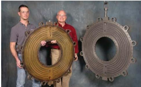
A new 36" composite water jacket (above, left) weighs approx. 95 lbs. A comparable 36" cast iron jacket (above, right) weighs approx. 375 lbs. The reduced weight is a significant maintenance and installation benefit in weight-restricted applications.
