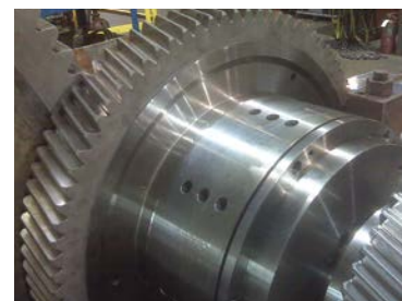
HC/CH clutches feature extra thick plates combined with high performance friction materials.
