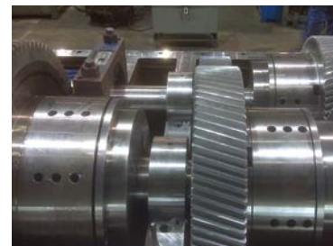
HC/CH clutches installed in drawworks gearbox.
