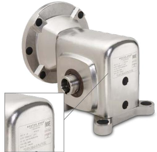
Laser marked nameplate provides worry-free part identification while maintaining a smooth, unetched surface. Rounded housing prevents foreign matter adherence and fluid accumulation.
