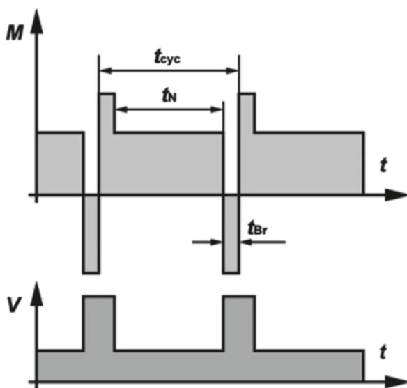
The machine starts up, operates under load, and then is braked electrically, for example by feeding it from a DC power source. Following this, it starts up again immediately. The machine can operate continuously in this manner if the specified moments of inertia of the motor *J<sub>M</sub>* and of the load *J<sub>ext</sub>* as well as the specified duty cycle are not exceeded. If the cycle duration is not specified, it is assumed to be 10 minutes.
