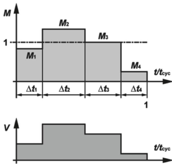
S10 duty comprises operation with at most four different load levels, each of which is maintained long enough to allow the machine to reach thermal equilibrium.
