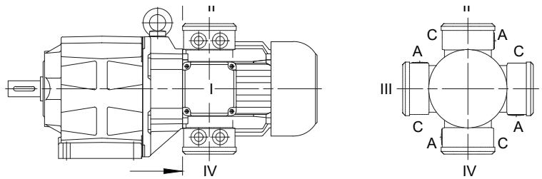
The standard position for the motor terminal box is shown in the dimensional drawings for the geared motors (see chapter 10, 11, 12 and 13). The terminal box can be installed at any of 3 other positions on request, if on-site space is restricted. The 4 possible positions are 90° offsets around the axis of the motor (dimensional drawing and designation for standard terminal box, see chapter 16 "Dimensional drawing standard terminal box").
