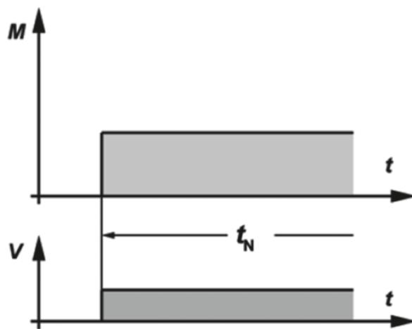
Operation under rated load for sufficient time to allow temperature equilibrium to be attained, such that the temperature does not increase any more with continued operation. The equipment can operate continuously under the rated load without exceeding the allowable temperature.
