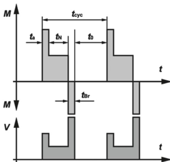
S5 duty consists of a sequence of identical cycles, each of which is composed of a starting time, a time of operation under constant load, a time of fast electric braking, and a rest period with the windings de-energised.
