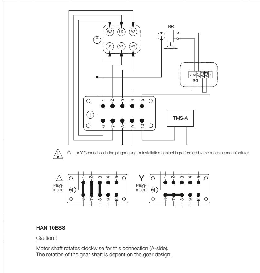
The motors are also available with a low-cost round plug connector as an alternative. This is fitted at the factory in the standard terminal box and is also suitable for brake connection, thermistors and thermostats. Additional information on request.
