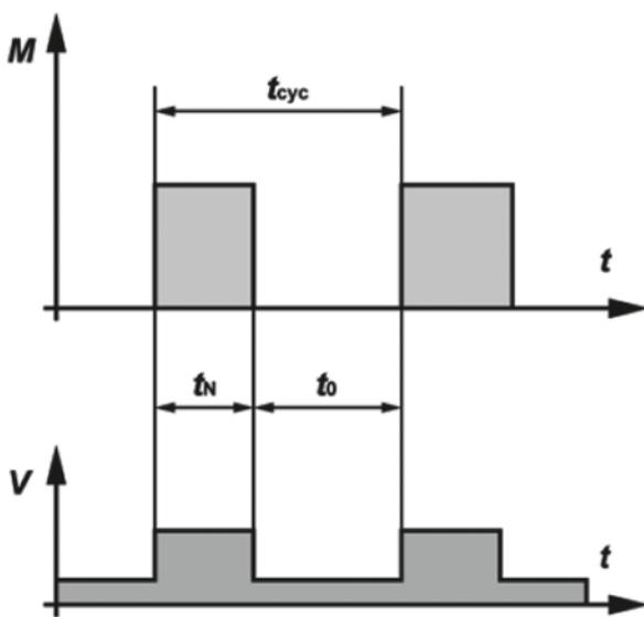
This type of duty corresponds to S3, with the exception that the equipment remains energised during the rest periods. In other words, it operates with no load during these periods. The duty cycle and cycle duration are specified the same way as for S3 duty.
