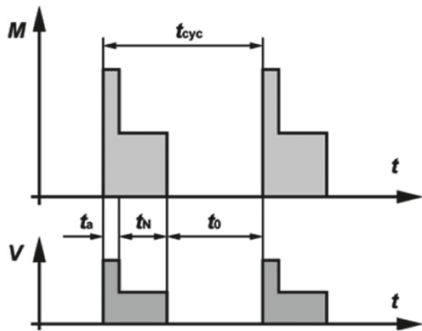
S4 duty consists of a sequence of identical cycles, each of which is composed of a distinct starting time, a time of operation under constant load, and a rest period with the windings de-energised.
