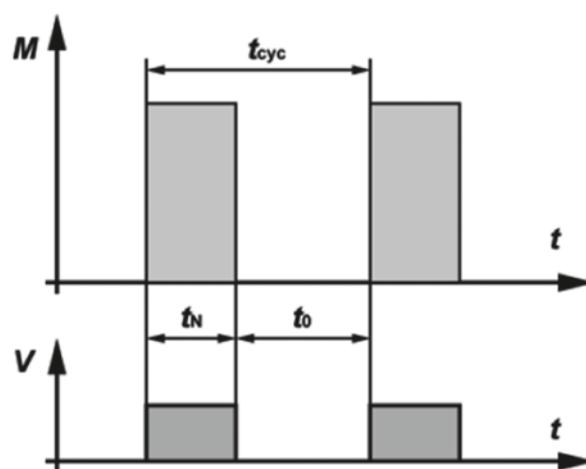
S3 duty consists of a sequence of identical cycles, each composed of an operating time with constant load and a rest time with the windings de-energised. The cycle is such that the starting current does not significantly affect the temperature rise. The operating time under rated load and the subsequent pause are both short. The equipment can operate under load only during the period indicated by the duty cycle as a percentage of the total cycle time (cycle duration).
