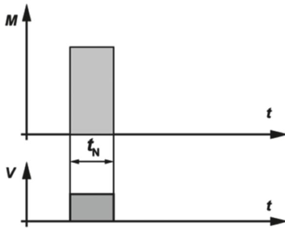
The operating time under rated load is short compared with the subsequent rest period. The standard operating times are 10, 30, 60 and 90 minutes. The equipment can operate for this period under the rated load without exceeding the allowable temperature.
