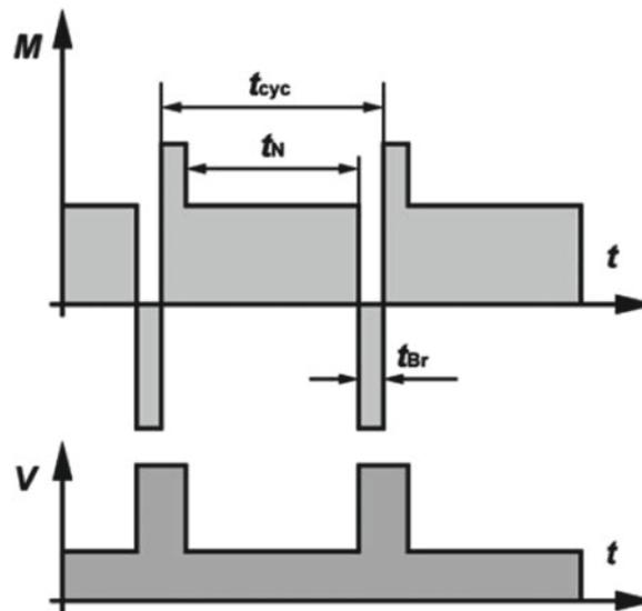
The machine starts up, operates under load, and then is braked electrically, for example by feeding it from a DC power source. Following this, it starts up again immediately. The machine can operate continuously in this manner if the specified moments of inertia of the motor  $J_M$  and of the load  $J_{Ext}$  as well as the specified duty cycle are not exceeded. If the cycle duration is not specified, it is assumed to be 10 minutes.
