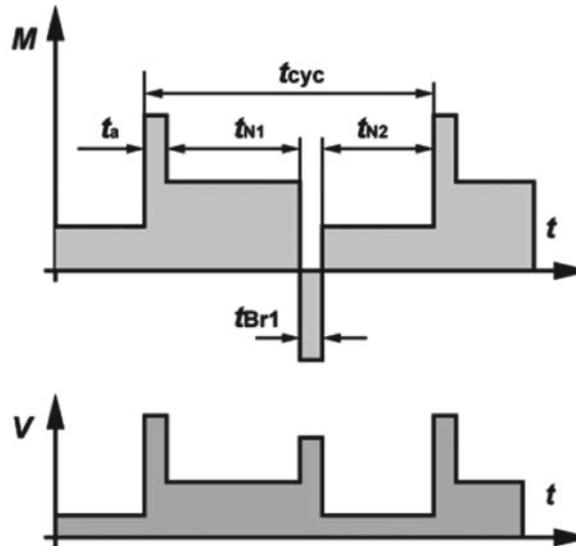
The machine runs continuously under variable load with frequent speed variations. The machine can operate continuously in this manner if at each speed the specified values are not exceeded (moments of inertia  $J_M$  and  $J_{Ext}$  cycle duration (if other than 10 minutes), rated output and duty cycle. With a moment of inertia of 1 kg m<sup>2</sup>, the acceleration characteristics are the same as with a mass of 1 kg at a distance of 1 m from the axis of rotation).
