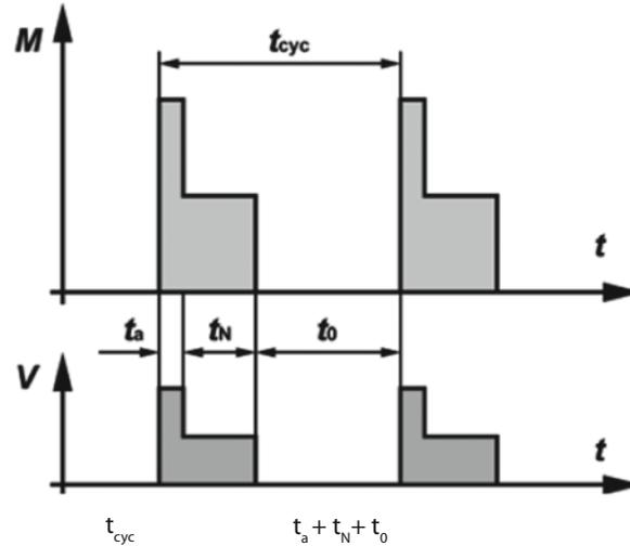
S4 duty consists of a sequence of identical cycles, each of which is composed of a distinct starting time, a time of operation under constant load, and a rest period with the windings de-energized.
