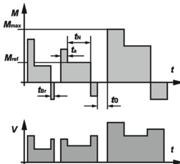
In S9 duty the load and the speed vary non-periodically within the permissible operating range. This includes frequently applied overloads, which must never exceed the reference load.
