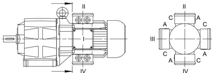
The standard position for the motor terminal box is shown in the dimensional drawings for the geared motors (see chapter 10, 11, 12 and 13). The terminal box can be installed at any of 3 other positions on request, if on-site space is restricted. The 4 possible positions are 90° offsets around the axis of the motor (dimensional drawing and designation for standard terminal box, see chapter 17 "Dimensional drawing standard terminal box").
