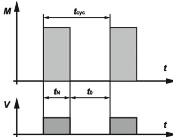
S3 duty consists of a sequence of identical cycles, each composed of an operating time with constant load and a rest time with the windings de-energized. The cycle is such that the starting current does not significantly affect the temperature rise. The operating time under rated load and the subsequent pause are both short. The equipment can operate under load only during the period indicated by the duty cycle as a percentage of the total cycle time (cycle duration).
