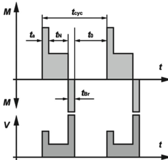
S5 duty consists of a sequence of identical cycles, each of which is composed of a starting time, a time of operation under constant load, a time of fast electric braking, and a rest period with the windings de-energized.
