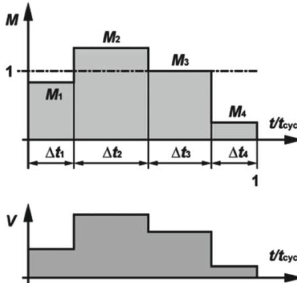
S10 duty comprises operation with at most four different load levels, each of which is maintained long enough to allow the machine to reach thermal equilibrium. The minimum load within a duty cycle may have a value of zero (no-load operation or at rest with the windings de-energized).
