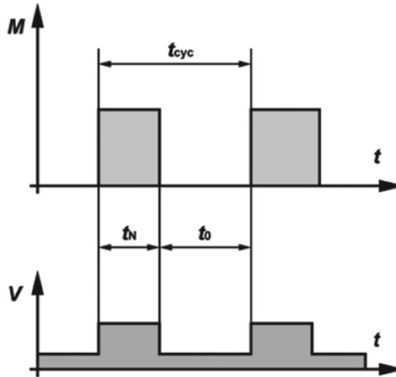
This type of duty corresponds to S3, with the exception that the equipment remains energized during the rest periods. In other words, it operates with no load during these periods. The duty cycle and cycle duration are specified the same way as for S3 duty.
