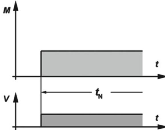
Operation under rated load for sufficient time to allow temperature equilibrium to be attained, such that the temperature does not increase any more with continued operation. The equipment can operate continuously under the rated load without exceeding the allowable temperature.
