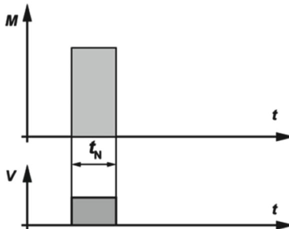
The operating time under rated load is short compared with the subsequent rest period. The standard operating times are 10, 30, 60 and 90 minutes. The equipment can operate for this period under the rated load without exceeding the allowable temperature.
