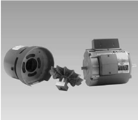
Kit includes all of the components needed for conversion of a 56C or 143-5TC frame totally enclosed fan cooled motor\* to a brakemotor. (Totally enclosed Stearns brake, replacement cast fan cover, shaft extension and fan/hub.) Mounts on fan end of motor. May be used on single or three phase motors.
