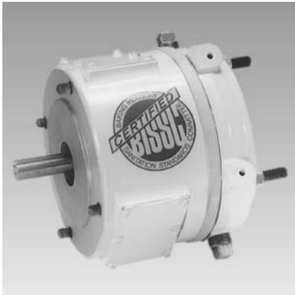
Double C-Face brakes provide the simplest solution for adding a brake between a C-Face motor and a flanged gear reducer. These brakes offer the added feature of meeting BISSC standards, AAA standards and other food industry washdown requirements. The CMB-WB double C-Face brakes are a perfect compliment to our AC washdown motors.
