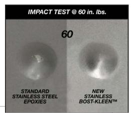
The QC700 Series is also available with a number of options including Bost-Kleen™ and Stainless Bost-Kleen™ washdown duty coatings, stainless steel output shafts and the award-winning PosiVent® pressure equalization system.
