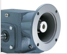
This smooth, clean motor flange dramatically improves any washdown application. The elimination of the coupling alignment hole ensures that debris and bacteria will not collect on this reducer.
