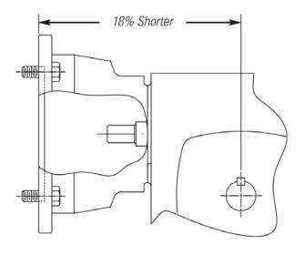
Along with these innovative product features, the gearboxes are significantly shorter (18% on average) than standard coupling mounted worm reducers on the market.
