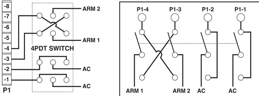
**Connection for RBD Series:** The customer provides interconnecting wiring.
