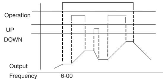
13. 5-00-06=16 (Principal/Auxiliary speed toggle) Multifunction terminal = OFF, the frequency is set by the VR (Master Speed) on the Keypad. While, Multifunction terminal = ON, the frequency is set by the analog signal terminal (Auxiliary Speed) on the TM2 on terminal Block.
