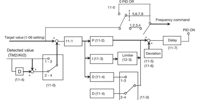
1. Performing PID control, set parameter 5-05=23, AV2 to TM2 as PID feedback signal.
