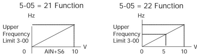
19. 5-00~06=23 (Analog Input AIN) The multifunction terminal AIN=23. The action is provided for setting the frequency.
