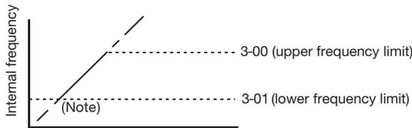
**\*Note:** When 3-01 = 0Hz and frequency command is 0Hz, the drive will stop at zero speed. When 3-01 > 0Hz and frequency command  $\geq$ 3-01, the drive will output parameter 3-01 value.
