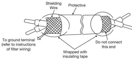
For 230V class ground 100Ω or less; for 480V class ground 10Ω or less.
