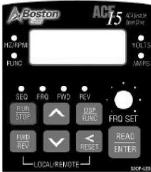
1. **Hz/RPM LED** – Indicates Speed Reference (Frequency) when stopped and Output Frequency when running. To display RPM, or Engineering units it must be selected in the program. See parameters 4-04 and 4-05 on page 36.
