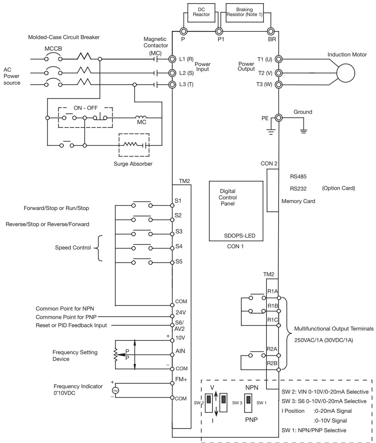
**Note 1:** Please refer to description of main circuit terminals (P1, BR) and specification of braking resistor for value selection. (Table 6.2 Dynamic Braking Resistor)
