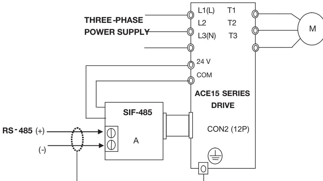
**Note:** Please put on the cover of drive to avoid the Interface Card disturbed by outside static electricity.
