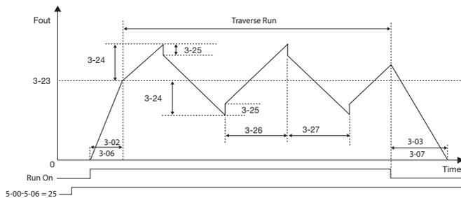
2. During traverse run, the center frequency could be controlled by the multifunction input terminals. However, the X upper deviation and Y lower deviation cannot be input at the same time. If they are inputted at the same time, the drive will maintain the original center frequency. The motion is as the graph below:
