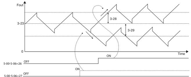
3. The stall prevention is idle during the acceleration and deceleration time of traverse run. Whereas, it is valid during first acceleration to center frequency process when the Function of traverse run is OFF or the drive is in deceleration time after the STOP command is received.
