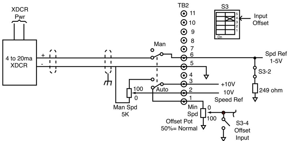
Figure 16. Signal Connection Diagram, 4-20 mA Transducer with Auto/Manual Switch
