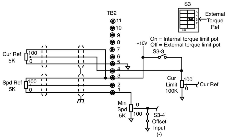
Figure 13. Signal Connection Diagram, Current (Torque) Reference Potentiometer
