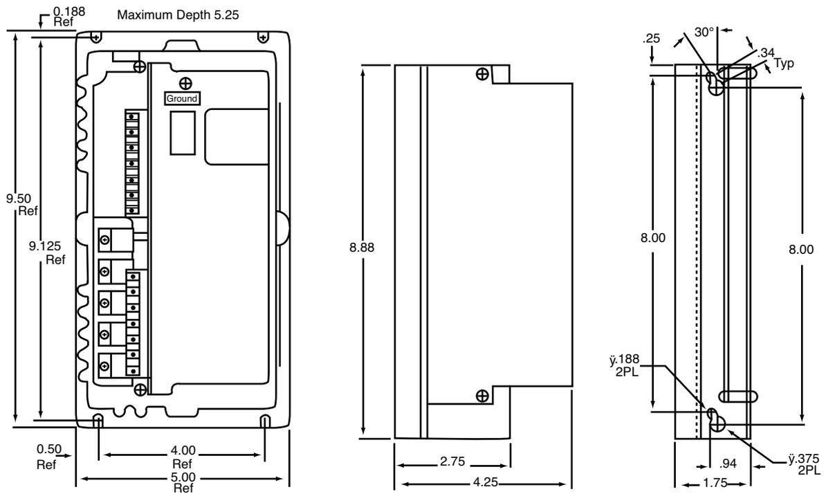
Figure 2. Controller Mounting Dimensions
