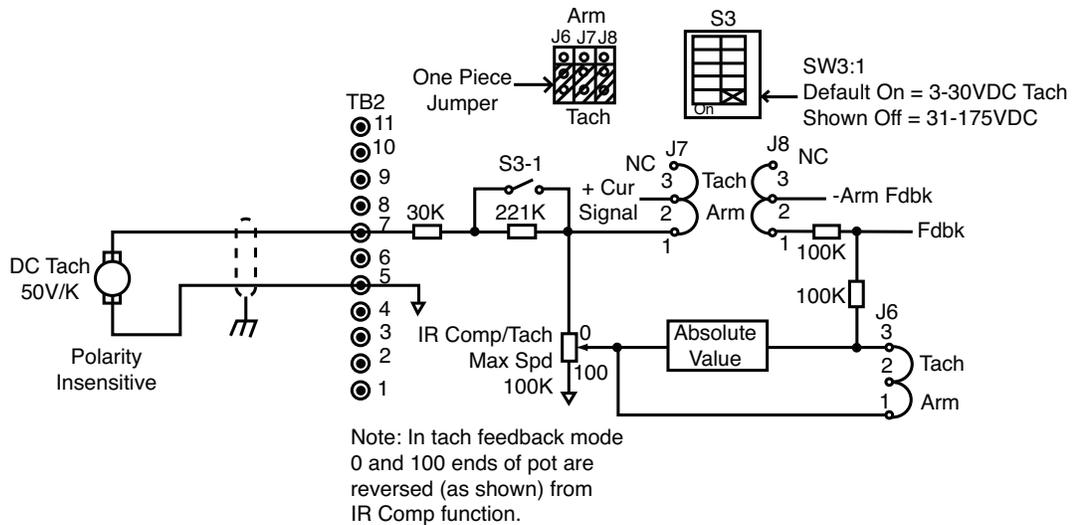
Figure 12. Signal Connection Diagram, Tachometer Feedback
