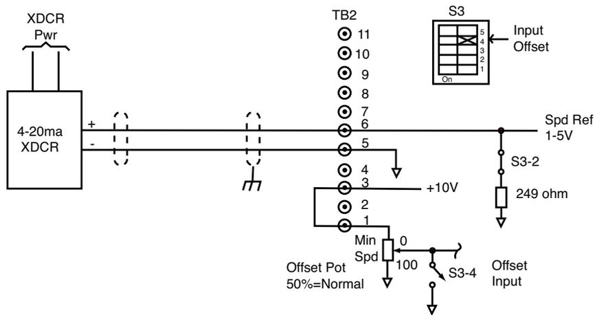
Figure 15. Signal Connection Diagram, 4-20 mA Interface
