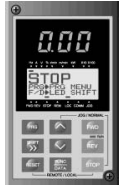
Fig. 3-1-2 Display on keypad panel at power-on
