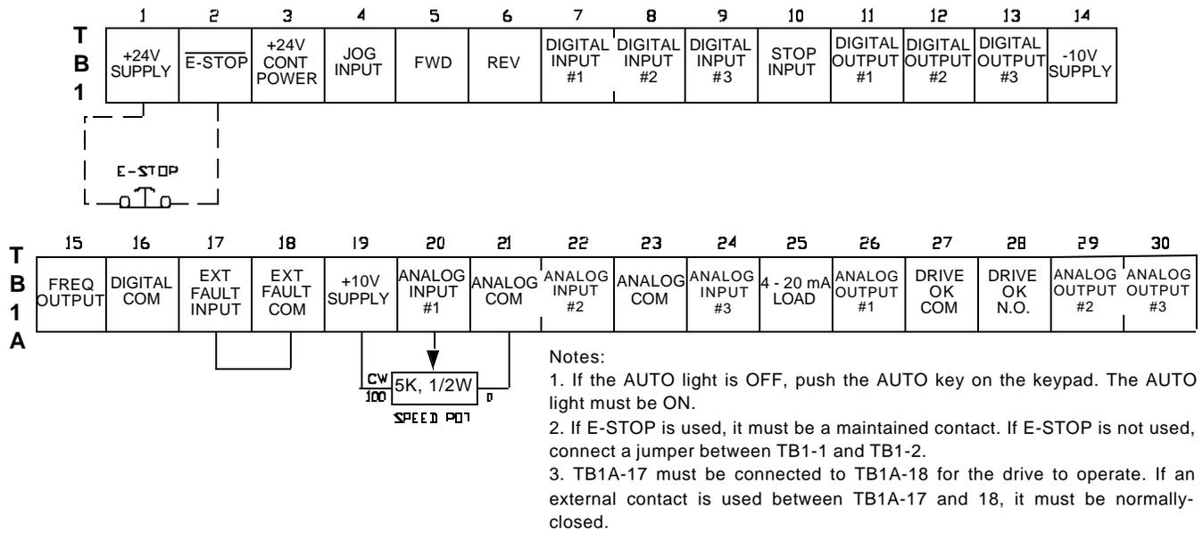
**FIGURE 6 - 1. WIRING DIAGRAM, SPEED CONTROL POT - KEYPAD OPERATION**
