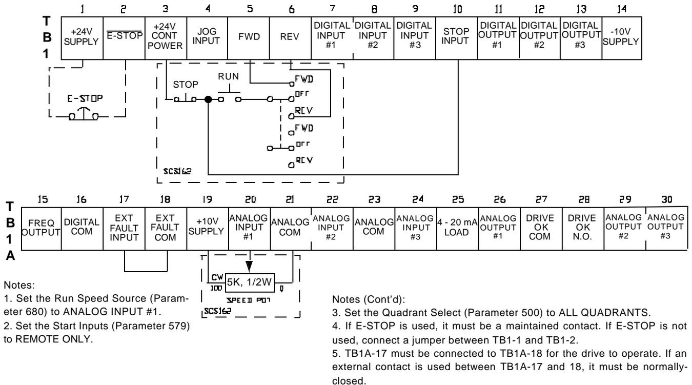
FIGURE 6 - 8. WIRING DIAGRAM, BOSTON GEAR RCS2A REMOTE STATION (RUN & STOP BUTTONS, FORWARD/REVERSE SWITCH, & SPEED CONTROL POT) - REMOTE OPERATION
