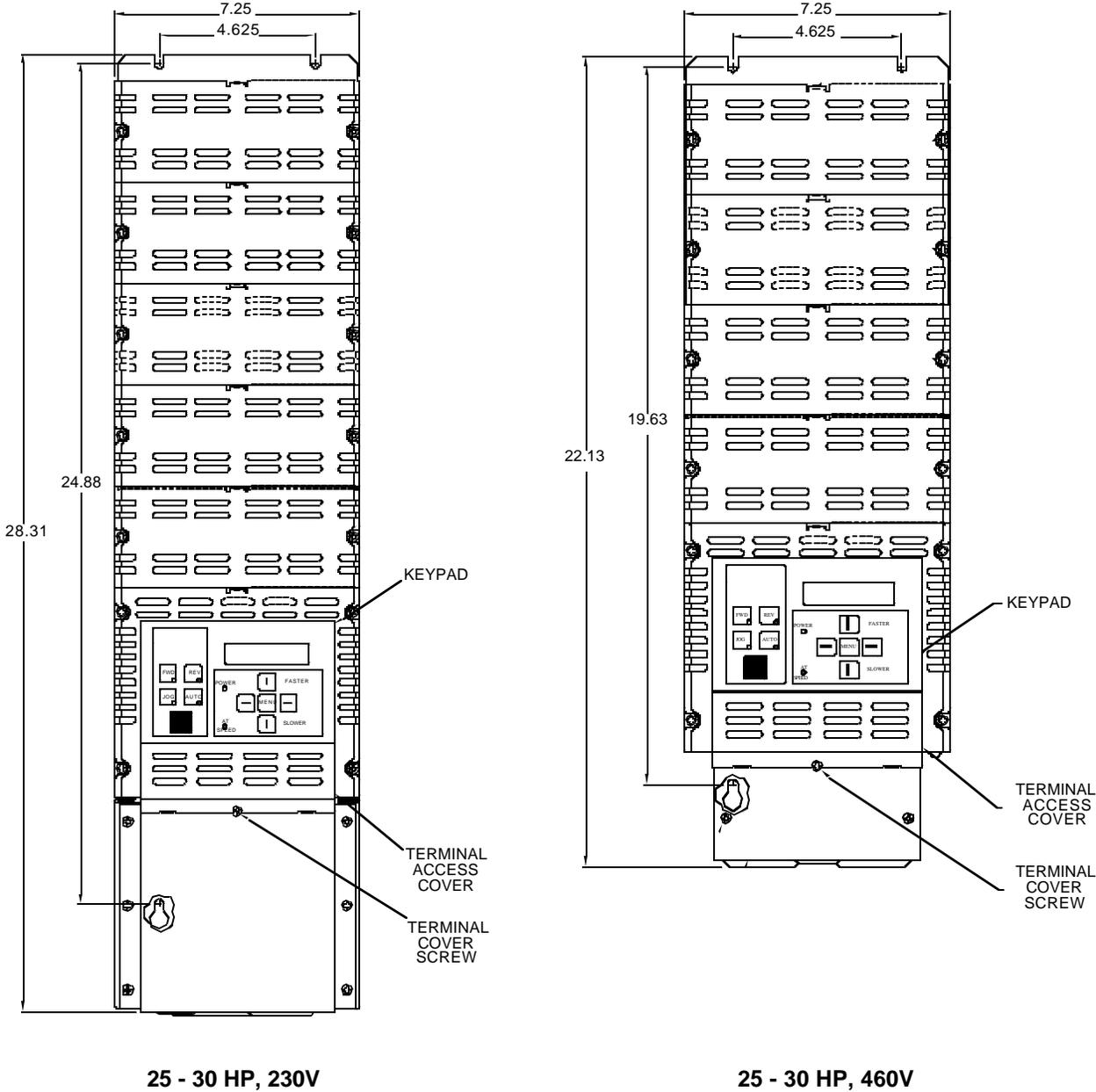
FIGURE 2-3. ADX CONTROLLER MOUNTING DIMENSIONS, 25 - 30HP, 230/460V
