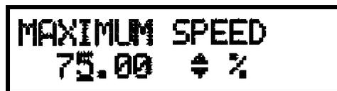
To enter the 75% maximum speed into the controller memory, push the MENU key. The display should read as follows:
