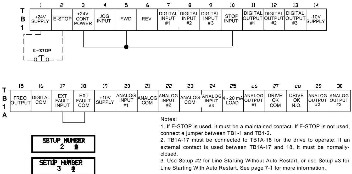
**FIGURE 7 - 2. WIRING DIAGRAM FOR SETUP MODE #2 OR #3, LINE STARTING WITH OR WITHOUT AUTO RESTART**
