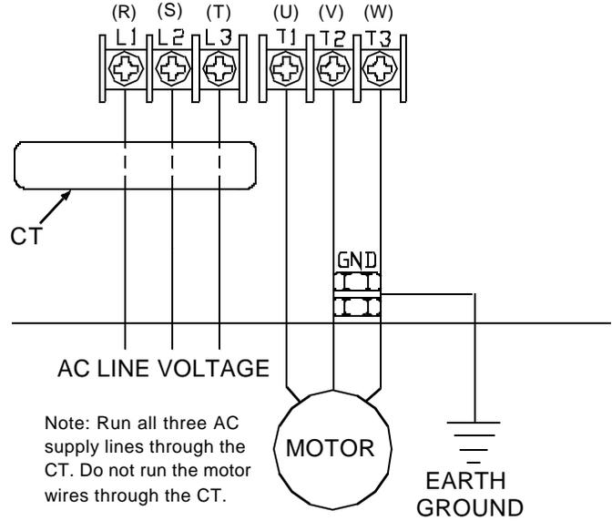
Note: Run all three AC supply lines through the CT. Do not run the motor wires through the CT.
