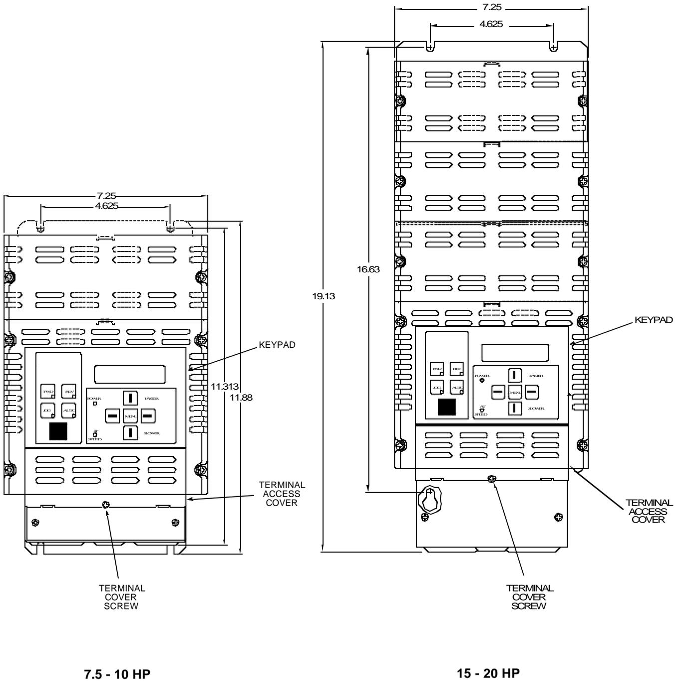
**FIGURE 2-2. ADX CONTROLLER MOUNTING DIMENSIONS, 7.5 - 20HP, 230/460V**
