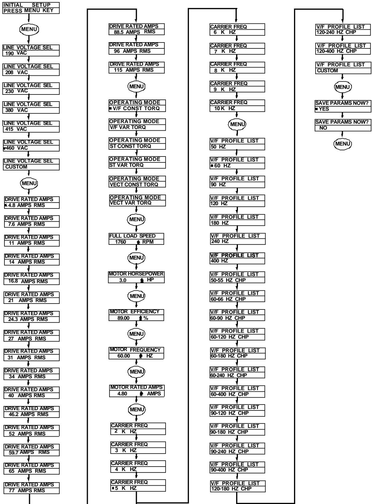
FIGURE 11 - 1. INITIAL SETUP FLOWCHART
