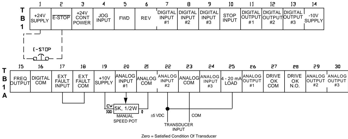
FIGURE 8 - 1. WIRING DIAGRAM, PID ERROR INPUT MODE CONNECTIONS
