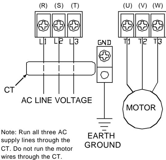
Note: Run all three AC supply lines through the CT. Do not run the motor wires through the CT.
