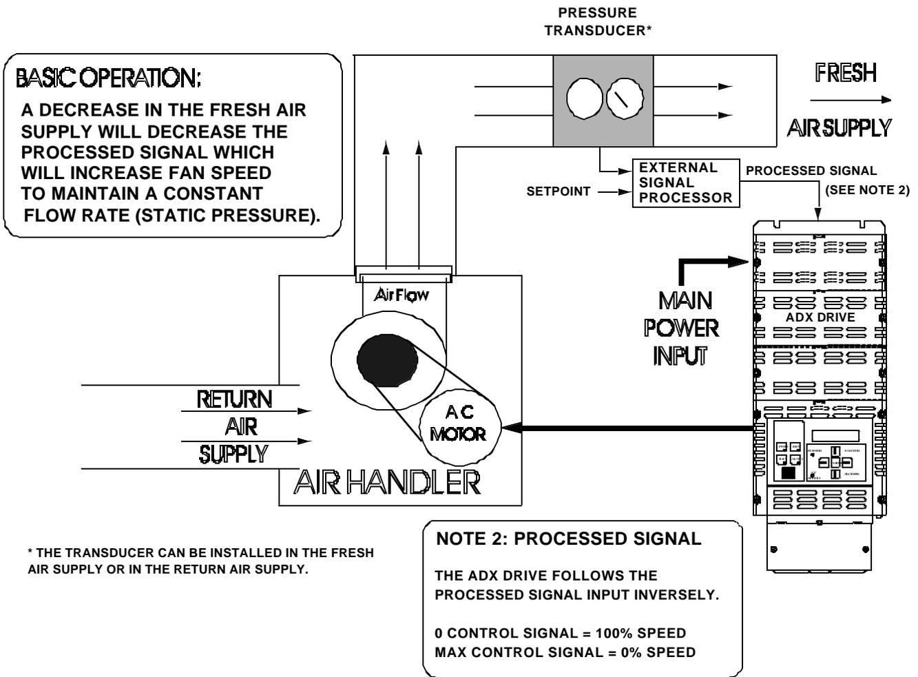
FIGURE 7-6. TYPICAL EXAMPLE OF AN AIR HANDLING APPLICATION USING INVERSE FOLLOWER CONTROL (SETUP #7)
