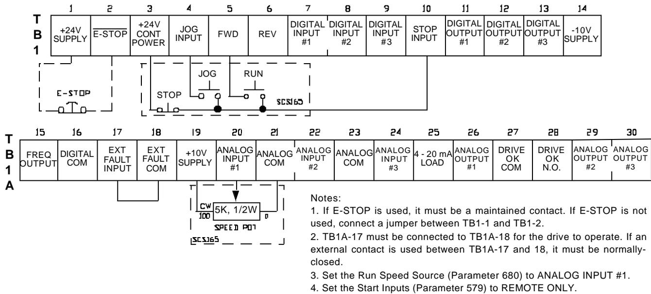
**FIGURE 6 - 9. WIRING DIAGRAM, BOSTON GEAR RCS5 REMOTE STATION (RUN, STOP & JOG BUTTONS, & SPEED CONTROL POT) - REMOTE OPERATION**
