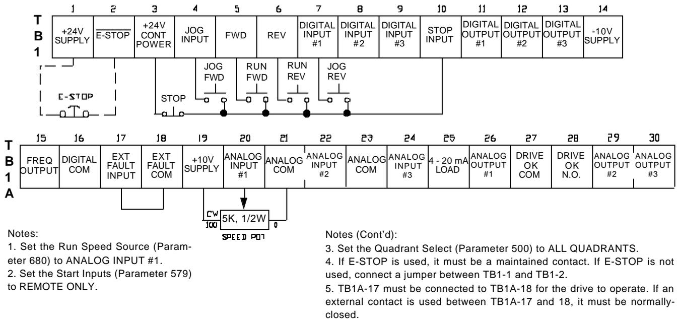
FIGURE 6 - 11. WIRING DIAGRAM, RUN FORWARD, RUN REVERSE, JOG FORWARD, JOG REVERSE & STOP BUTTONS, & SPEED CONTROL POT - REMOTE OPERATION
