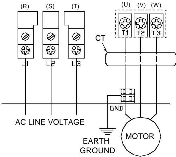
Note: Run all three motor wires through the CT. Do not run the AC supply lines through the CT.
