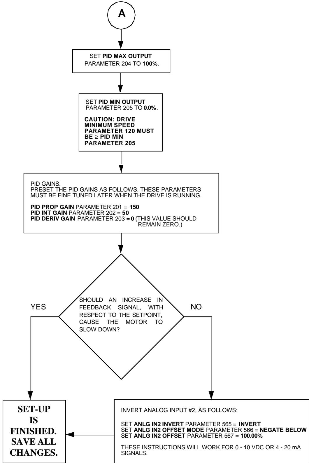
FIGURE 8 - 3. PID SET-UP FLOW CHART FOR PROCESS CONTROL (Cont'd)
