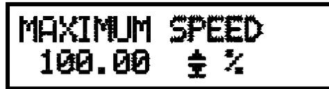
This display shows that maximum speed will be in percent. Its adjustment range, shown on page 4-7, is from 50.00% to 100.00% (equal to maximum frequency).
