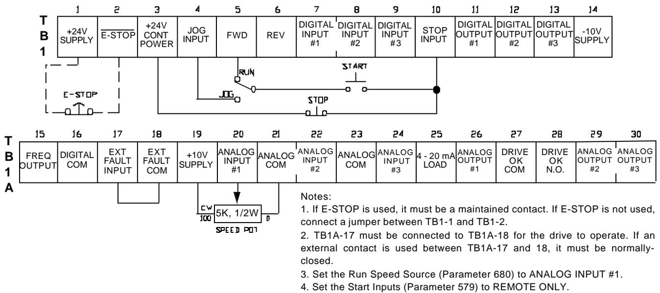
FIGURE 6 - 3. WIRING DIAGRAM, START & STOP BUTTONS, RUN/JOG SWITCH, & SPEED CONTROL POT - REMOTE OPERATION
