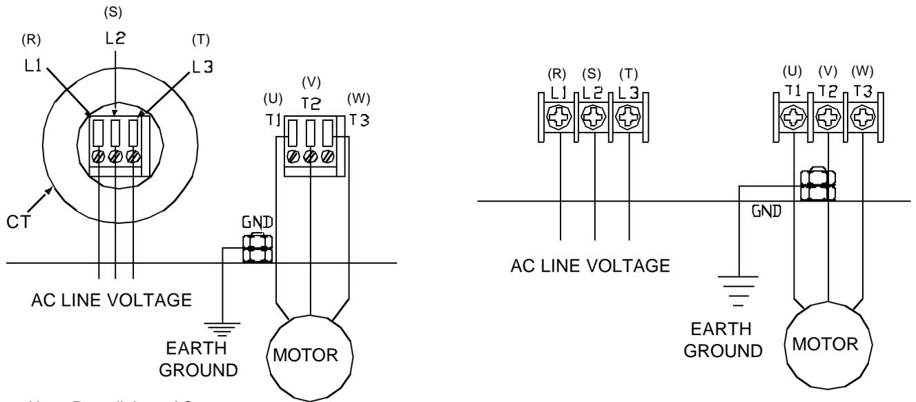
Note: Run all three AC supply lines through the CT. Do not run the motor wires through the CT.
