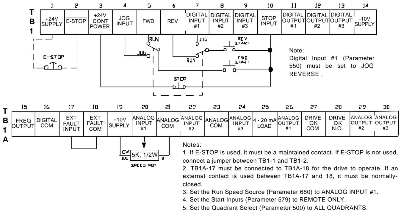
FIGURE 6 - 4. WIRING DIAGRAM, FORWARD, REVERSE & STOP BUTTONS, RUN/JOG SWITCH, & SPEED CONTROL POT - REMOTE OPERATION
