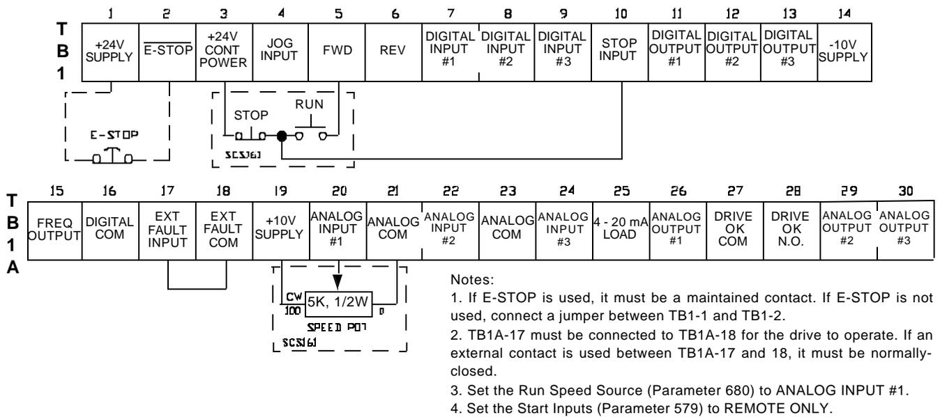
FIGURE 6 - 7. WIRING DIAGRAM, BOSTON GEAR RCS1 REMOTE STATION (RUN & STOP BUTTONS, & SPEED CONTROL POT) - REMOTE OPERATION
