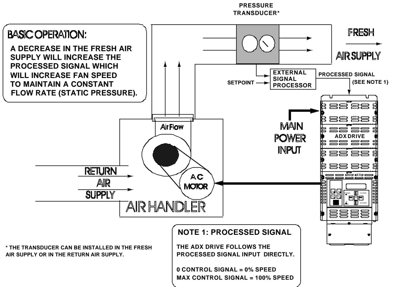
FIGURE 7-5. TYPICAL EXAMPLE OF AN AIR HANDLING APPLICATION USING DIRECT FOLLOWER CONTROL (SETUP #6)
