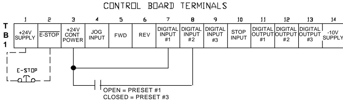
**WIRING DIAGRAM, TWO PRESET SPEEDS WITH ONE CONTACT**
