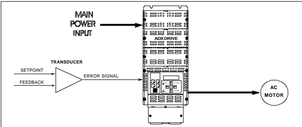
FIGURE 8 - 2. BLOCK DIAGRAM, PID ERROR INPUT MODE
