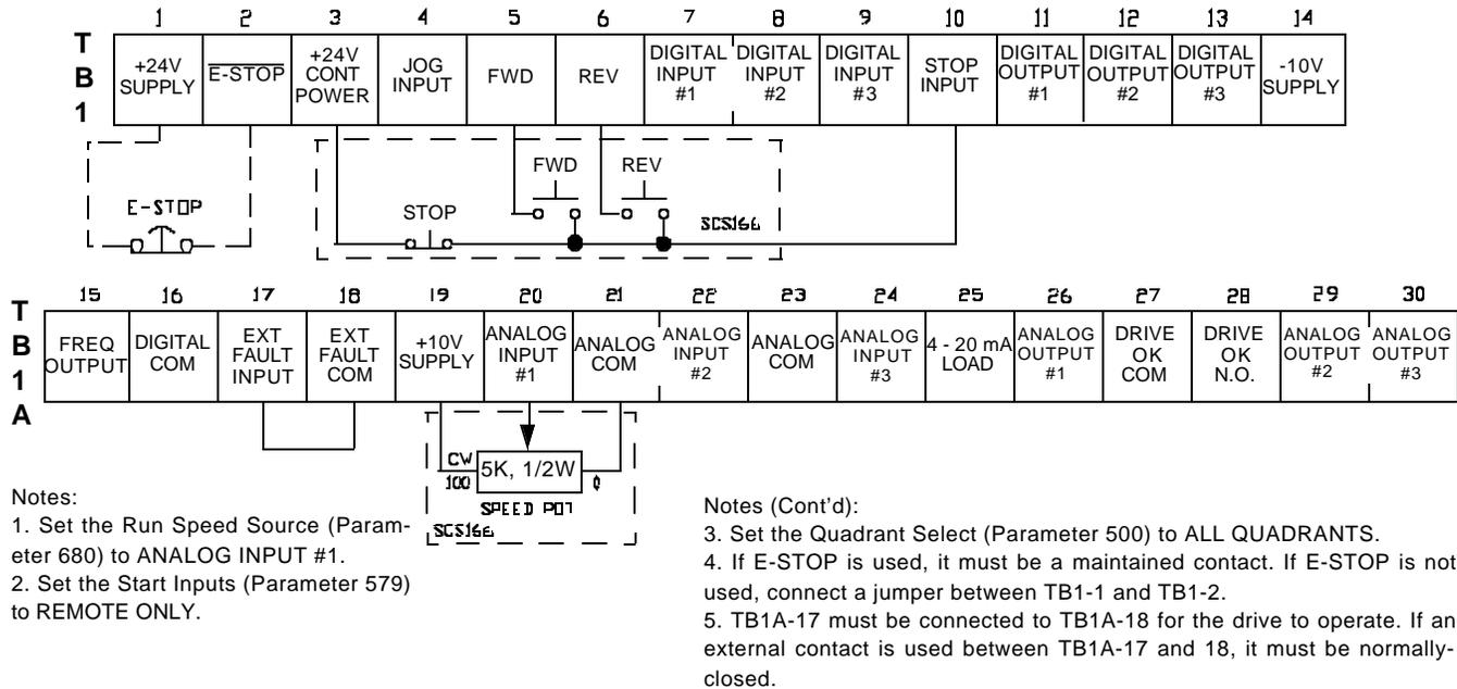
**FIGURE 6 - 10. WIRING DIAGRAM, BOSTON GEAR RCS6 REMOTE STATION (FORWARD, REVERSE & STOP BUTTONS, & SPEED CONTROL POT) - REMOTE OPERATION**
