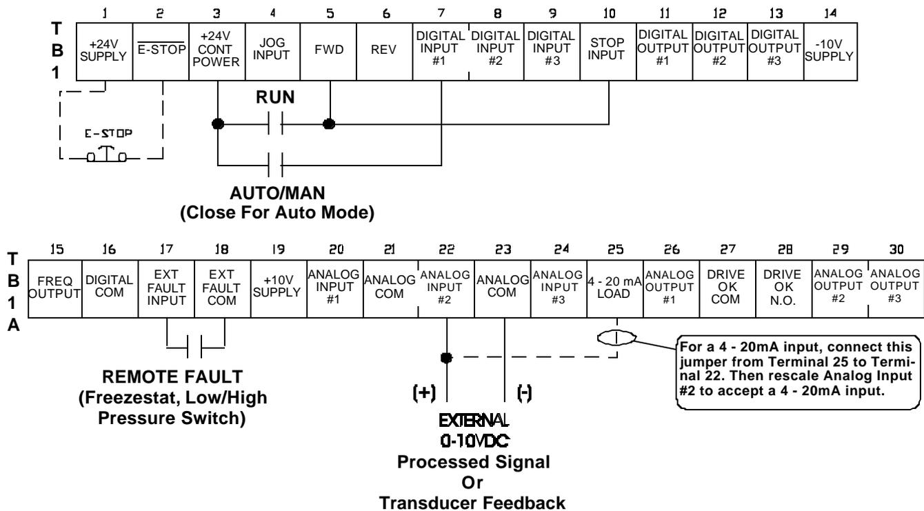
**FIGURE 7-10. TYPICAL WIRING DIAGRAM FOR APPLICATIONS WITH DIRECT FOLLOWER CONTROL (SETUP #6), INVERSE FOLLOWER CONTROL (SETUP #7), DIRECT PID CONTROL (SETUP #8 OR #10), OR INVERSE PID CONTROL (SETUP #9 OR #11)**
