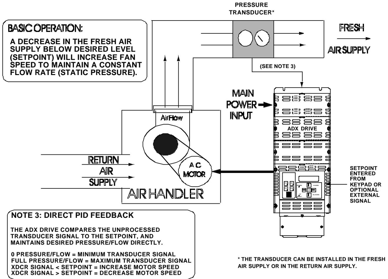
FIGURE 7-7. TYPICAL EXAMPLE OF AN AIR HANDLING APPLICATION USING DIRECT PID CONTROL (SETUP #8 OR SETUP #10)
