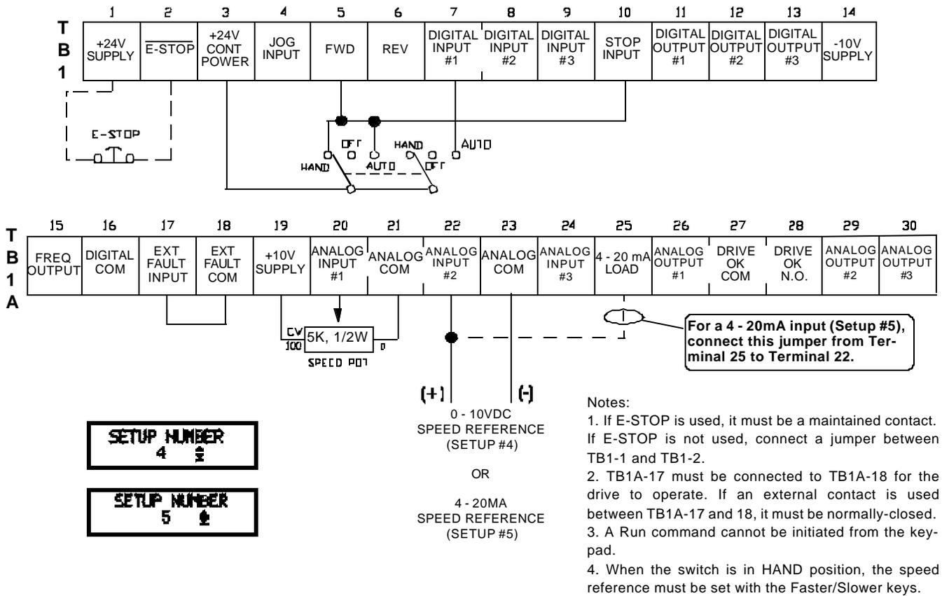
**FIGURE 7 - 3. WIRING DIAGRAM FOR SETUP MODE #4 OR #5, HAND/OFF/AUTO SWITCH WITH 0-10 VDC OR 4-20MA SPEED REFERENCE - REMOTE OPERATION**
