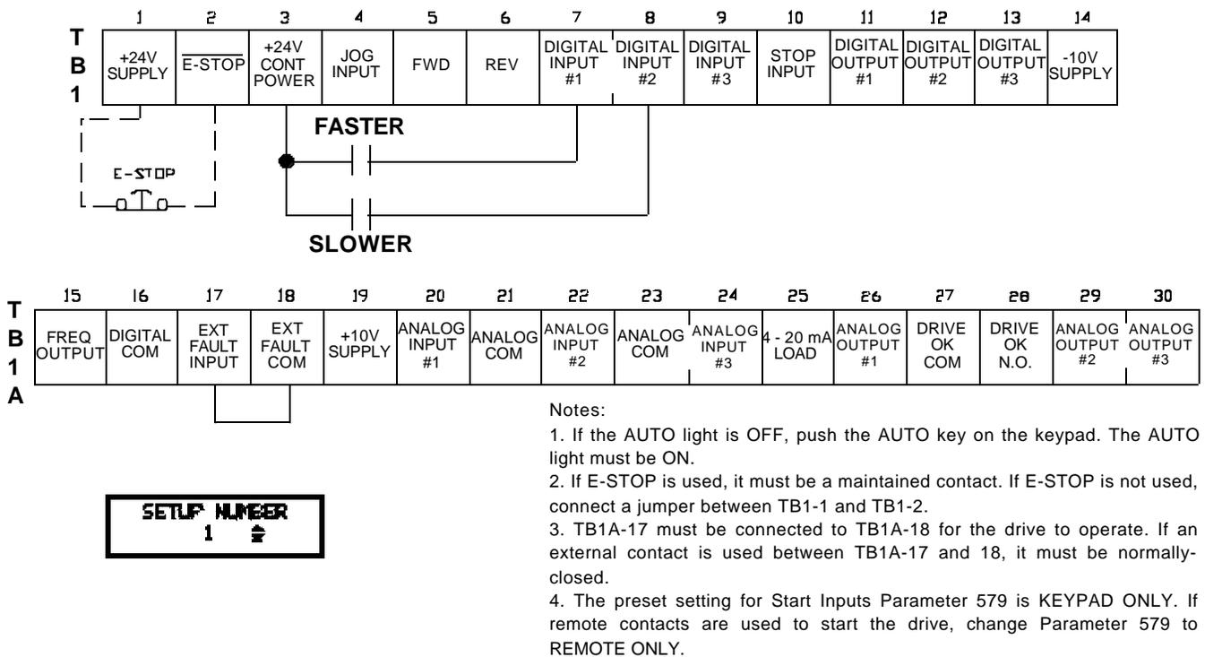
**FIGURE 7 - 1. WIRING DIAGRAM FOR SETUP MODE #1, FASTER/SLOWER - KEYPAD OR REMOTE OPERATION**
