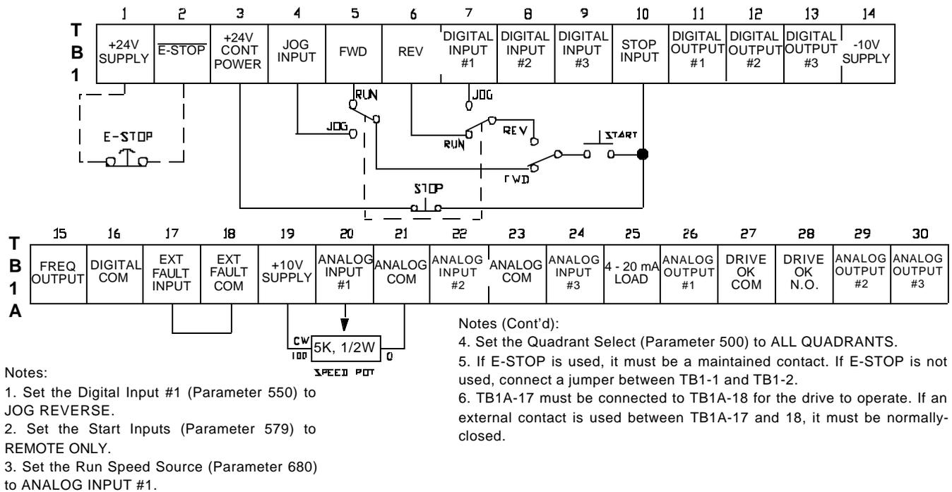
**FIGURE 6 - 6. WIRING DIAGRAM, START & STOP BUTTONS, FORWARD/REVERSE & RUN/JOG SWITCHES, & SPEED CONTROL POT - REMOTE OPERATION**
