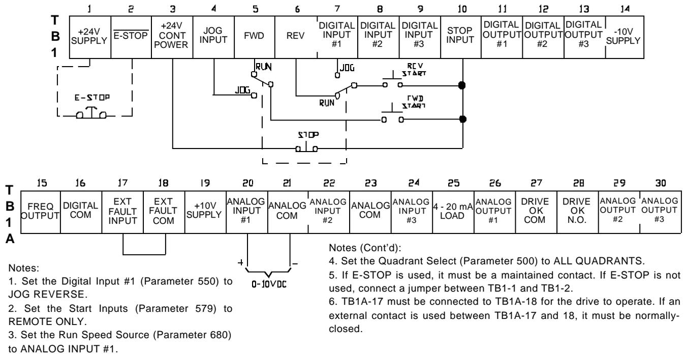
**FIGURE 6 - 5. WIRING DIAGRAM, FORWARD, REVERSE & STOP BUTTONS, RUN/JOG SWITCH, & 0 - 10 VDC SPEED REFERENCE SIGNAL - REMOTE OPERATION**
