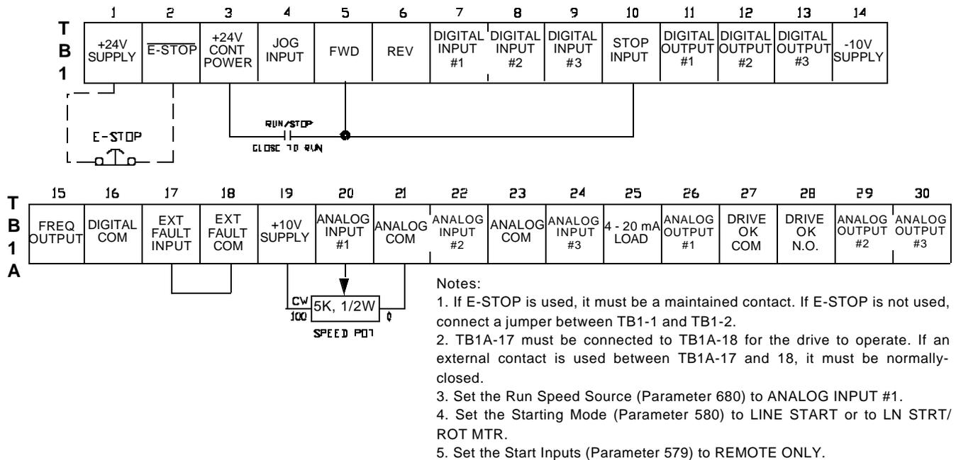
**FIGURE 6 - 2. WIRING DIAGRAM, TWO-WIRE START/STOP & SPEED CONTROL POT - REMOTE OPERATION**
