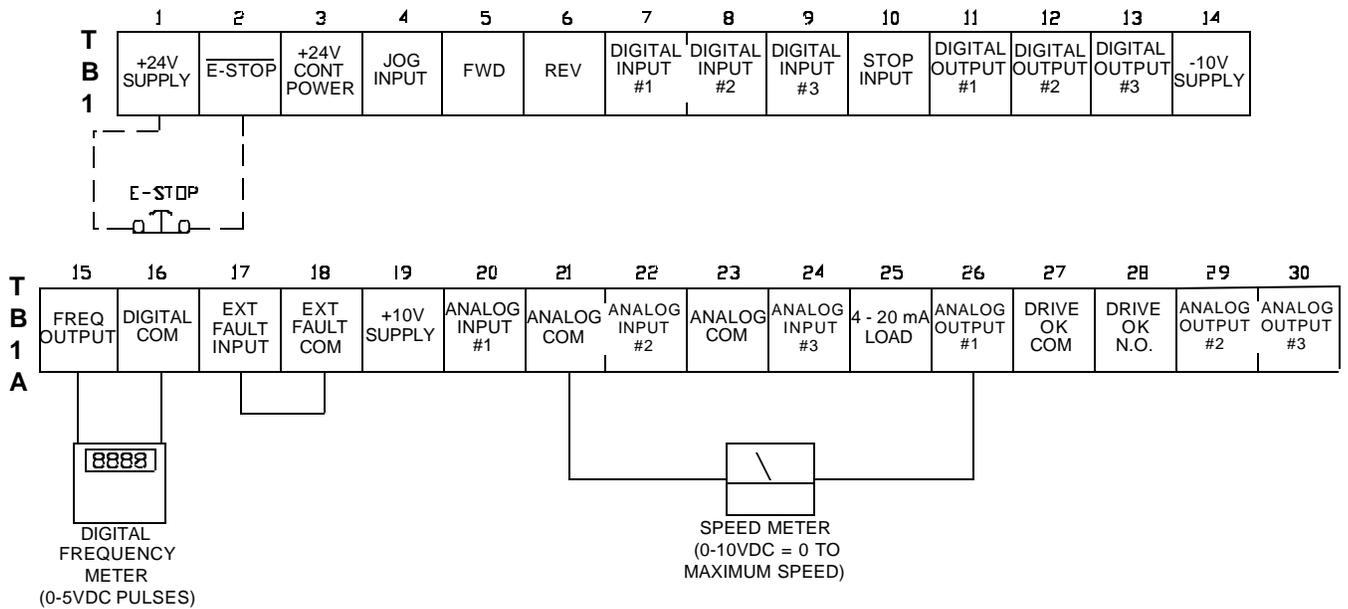
FIGURE 6 - 12. WIRING DIAGRAM, FREQUENCY & SPEED METERS - KEYPAD OR REMOTE OPERATION
