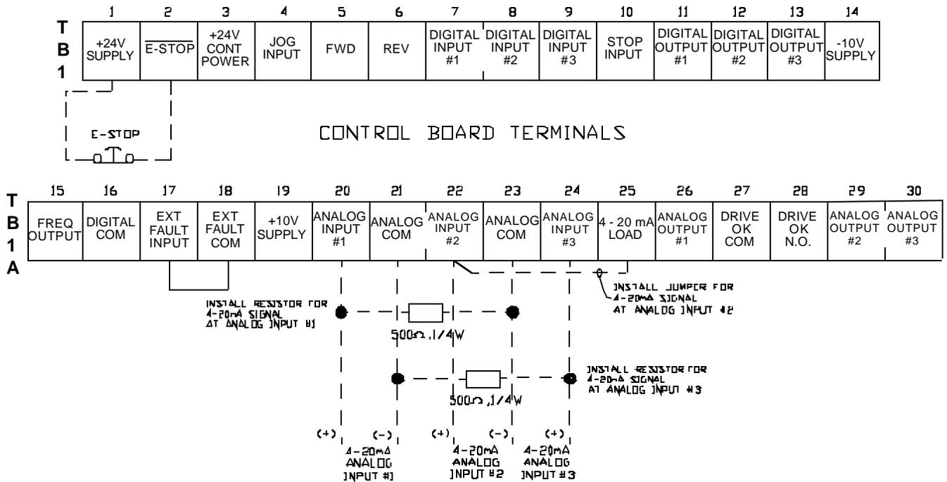
**WIRING DIAGRAM, ANALOG INPUTS**
