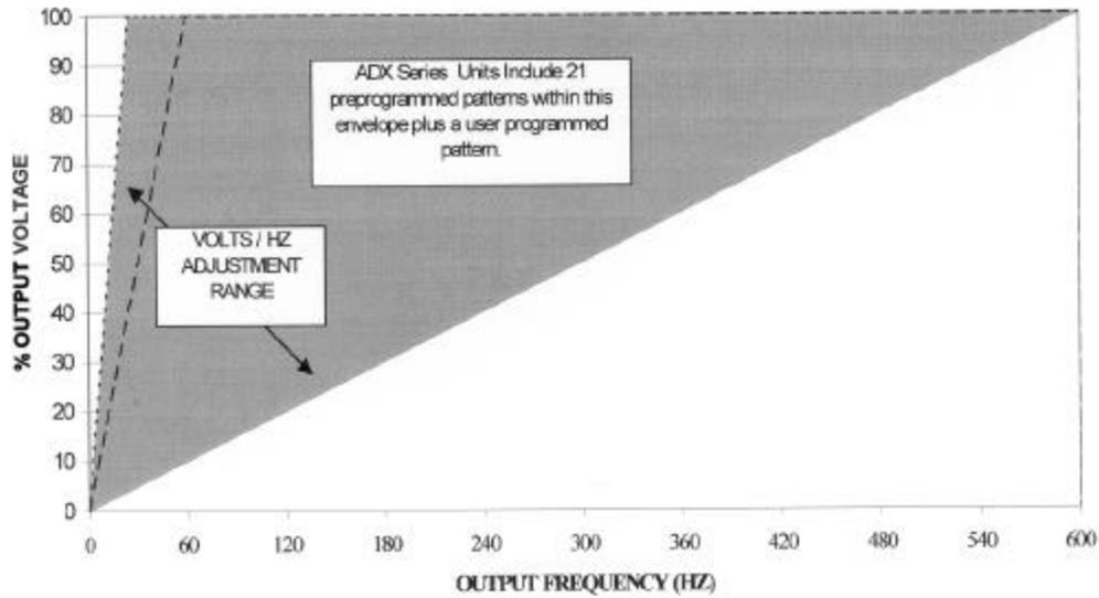
ADJUSTMENT RANGE FOR CONSTANT TORQUE APPLICATIONS.
