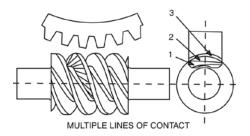
The involute helicoid ensures accuracy of profile and shape necessary to obtain proper contact and closeness of contact. More load carrying capacity, better accuracy, and longer life than any other thread form are assured. Note: above diagrams show 3 teeth in contact (1, 2, 3).
