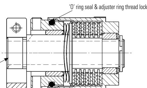
**Sectional view of 6-plate Vari-Tork Ref. 409.25 Shafts are secured by a split hub and ring clamp method which does not score the shafts.**
