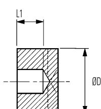
Controlled bore depth L1 provides a register when pre-assembling hubs to shafts
