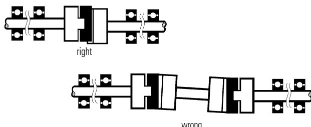
Note: It is important that installed couplings are not end-loaded. To help avoid this, thro' bored hubs are recommended for shafts which have fixed axial locations such as face-mounted motors.
