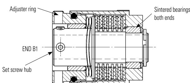
**Sectional view of 6-plate Vari-Tork Ref. 279.25 Shafts are secured by set screws accessed through radial holes in the adjuster ring.**
