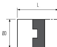
User-adaptable for special needs, e.g. fitting within tubes. Blank hubs are supplied centred with no provision for fastening. External dimensions identical with blind hubs.
