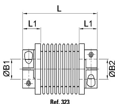
The convolutions of Flex-Ni Couplings are formed by the electrolytic deposition of nickel. This produces stress-free convolutions with closely controlled wall thickness.
