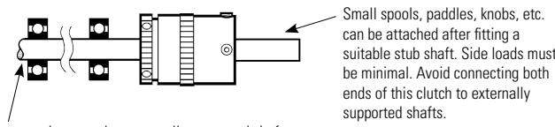
**BASIC CLUTCH + FLEXIBLE COUPLING - REFS. 267, 269, 277, 285, 397, 399, 407 & 415** Controlled slip occurs between LH & RH shafts.
