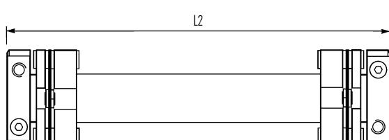
Unless specified otherwise, drive shafts are supplied with set screw hubs inboard.
