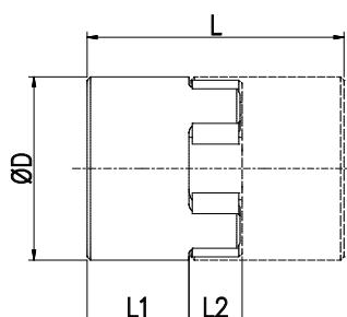
User-adaptable for special needs e.g. fitting within tubes. Blank hubs are supplied centred with no provision for fastening. External dimensions identical with blind hubs.
